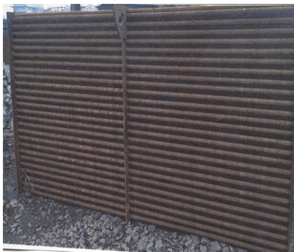
Figura 1 - General view of the top high-temperature section of heat exchanger to heat air
