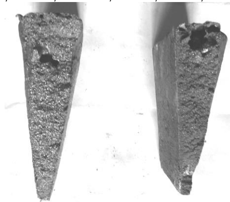
Figure 3 – Fracture of non-modified (on the left) and modified cast irons
