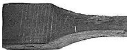
Figure 4 - An underrolled specimen of the lead alloy C1+3% Sb without defects after reduction \varepsilon > 60\% under conditions of limiting the strip shearing
